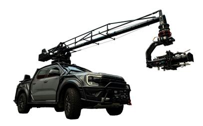
The Scorpio Arm is a different concept of Camera Car. With it we can do camera movements from a car controlled from inside driving at high speed and having images of more stables, dynamics, and with all safety measures for the members of the team.
